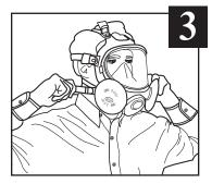
Tighten the two bottom straps.
