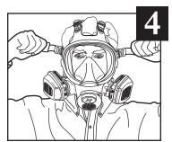
Tighten the two middle straps, then the two top straps.
