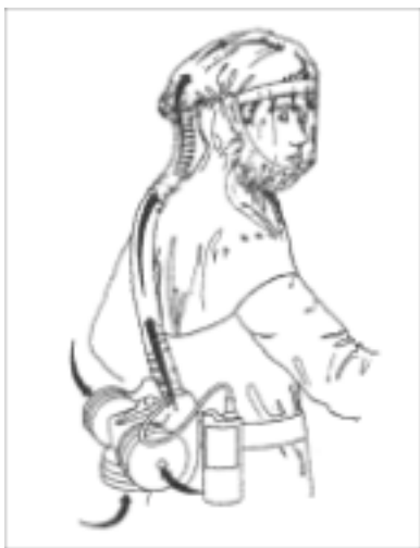
Fig. 1 3M™ R-Series Hood with Breathe Easy™ PAPR System
