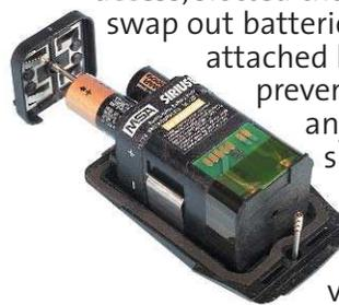
A lithium ion battery pack with optional vehicle charger is easily interchangeable with the alkaline battery pack. Charging the lithium ion battery pack can be done in the unit or
