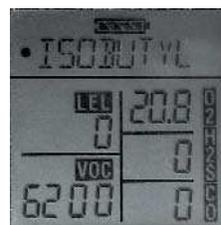
When measuring for general VOCs with isobutylene as the reference gas, users can easily read the chemical name "isobutyl" in a designated dashboard on the display. When a known gas is
