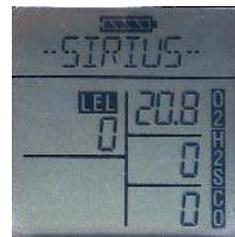
The Sirius Multigas Detector provides users outstanding multifunctional capabilities by integrating a high-performance PID (Photoionization Detector) sensor into a 4-gas detector. Users are able to simultaneously monitor for volatile organic compounds (VOCs) with low vapor pressures while measuring for combustible, toxic and oxygen-deficient atmospheres within one reliable, easy-to-use, durable unit.
