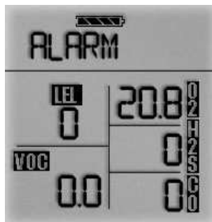
Figure 3-4b. Pump Alarm on the Display
