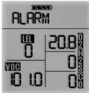
Figure 3-7b. Instrument in VOC Gas Alarm
