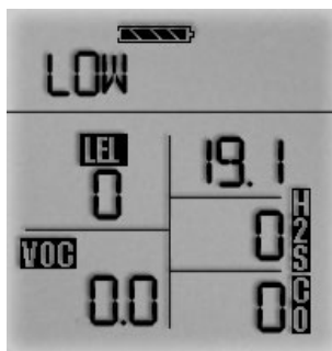
Figure 3-6a. Instrument in Oxygen Alarm
