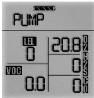
Figure 3-4a. Pump Alarm on the Display
